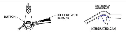
3. Turn cam arm adjustment nut inside cam arm yoke with fingers until it contacts surface of yoke. Turn outside nut with a 1 1/2" wrench tight against yoke to lock adjustment.
