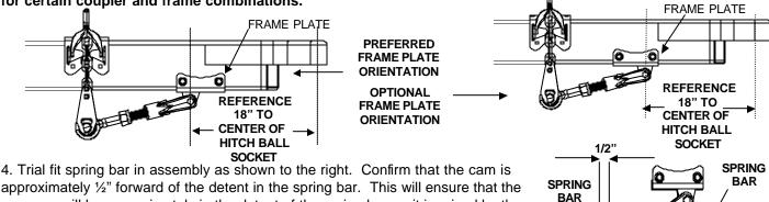
approximately ½" forward of the detent in the spring bar. This will ensure that the cam arm will be approximately in the detent of the spring bar as it is raised by the snap up bracket. It may be necessary to adjust frame plate position on frame for certain coupler and frame combinations.
