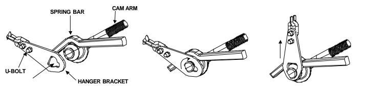
3. Before placing snap-up in position, ensure that the cam of the cam arm is about 1/2" forward of the bend in the spring bar, since the cam moves rearward as it is lifted by the snap-up bracket. After moving snap-up into the up position, install safety pin. Install second spring bar using the same number of chain links. Make sure that cams are mating each other properly.
